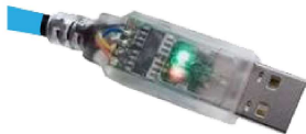
Figure 2: RS485 - USB for Orca GUI and firmware upgrades. This cable can also provide logic power
