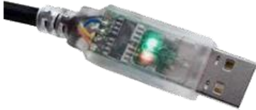
Figure 3: USB to RS485 for Orca motor GUI and firmware upgrades
